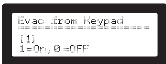
Figure 65. Evacuation from Keypad activation screen
